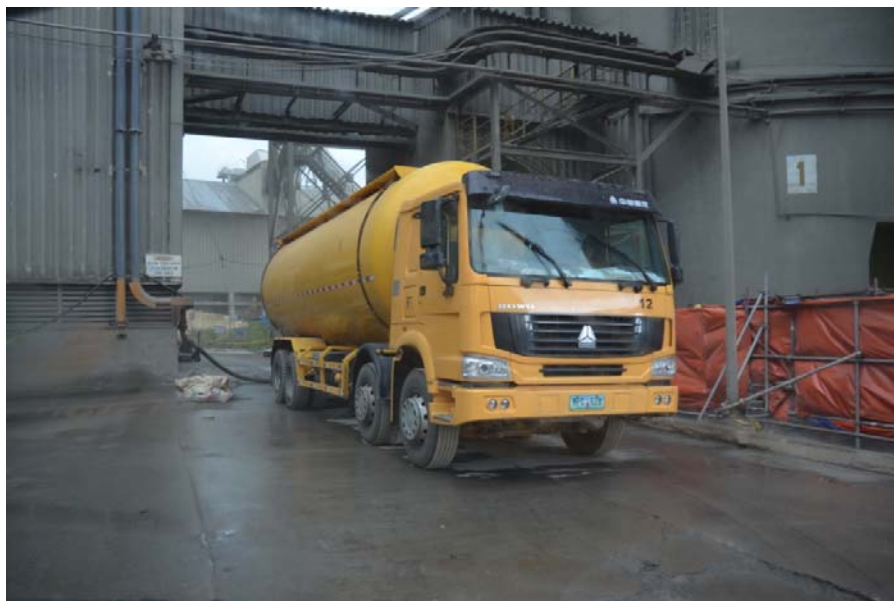
Figure 1: Covered Truck Unloading KSPC Fly Ash at APO Cement Facilities
